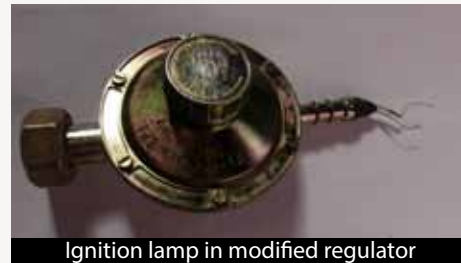
Ignition lamp in modified regulator
